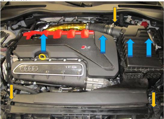
2. Unplug the MAP sensor, TPS sensor and undo the T30 torx fastener that holds the engine cover bracket and the stock dump valve. Then undo the hose clamp that holds the boost hose to the cast elbow.
